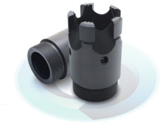
Material: 4140 75K PSI Ø 6" [152.4 mm] L 7" [177.8 mm] Special Processes: Molybdenum disulfide
